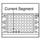
cline settings are not shown in the matrix.) To program a speed setting and an incline setting for the first segment, simply adjust the speed and incline of the treadmill as desired by pressing the Speed and Incline buttons. Every few times a Speed button is pressed, an additional indicator will light or darken in the Current Segment column.
